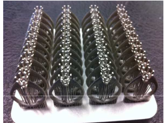
40 finished part with supports on platform are completed in 15 hours.
